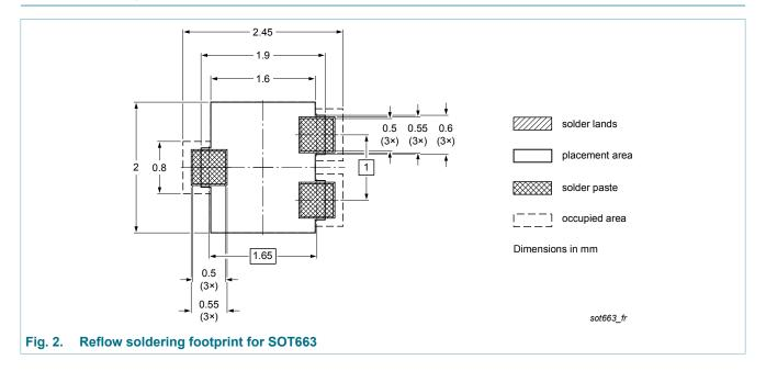
plastic, surface-mounted package; 3 leads; 1 mm pitch; 1.6 mm x 1.2 mm x 0.55 mm body
